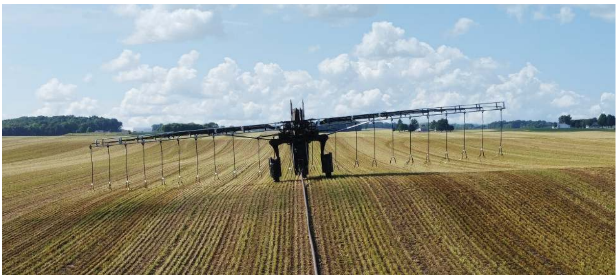
POWERFUL ELECTRIC MOTORS & A LOW CENTER OF GRAVITY GIVE 360 RAIN SOLID PERFORMANCE ON HILLS & SIDE SLOPES
